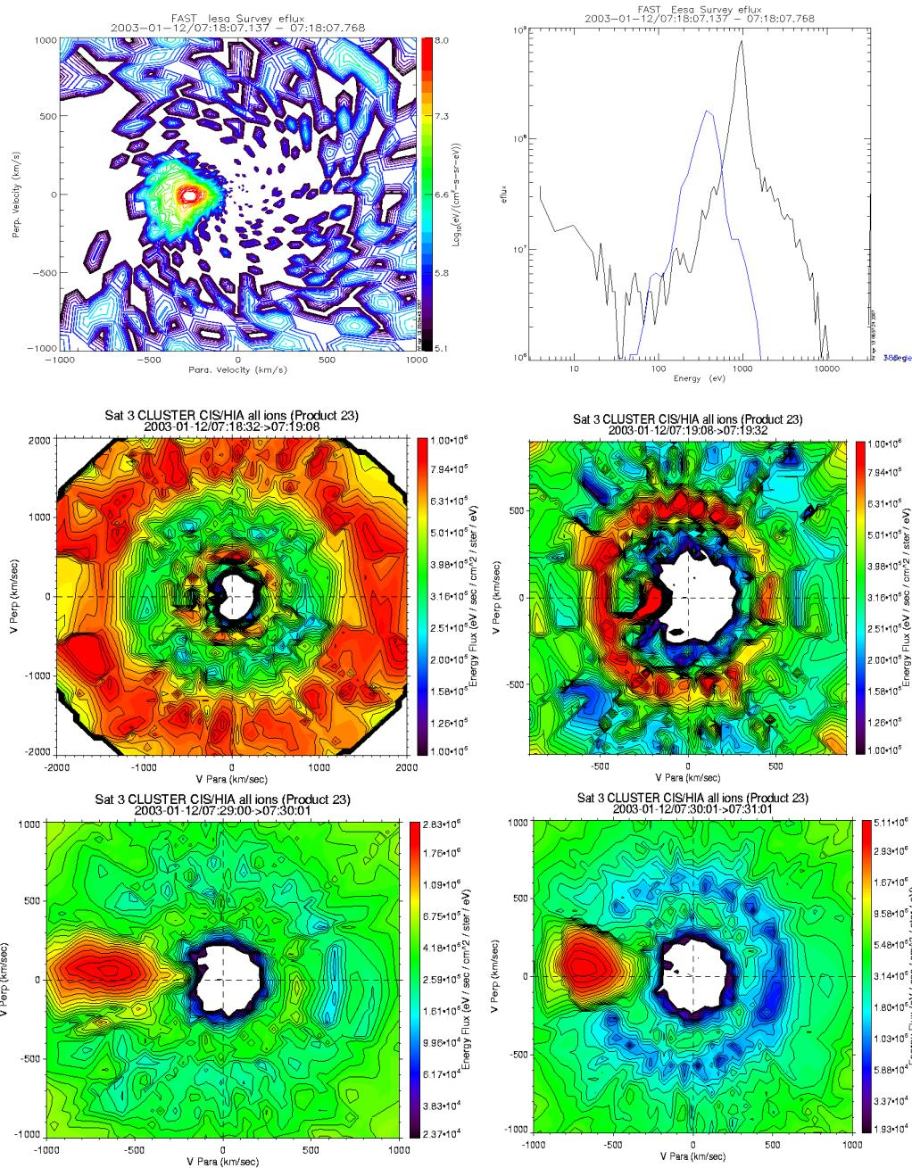
**Line 1:** FAST ion distribution (left) and electron/ion spectra (right). The data indicate a potential drop above the satellite of about 1 keV, and below the satellite of about 0.4 keV, providing a total of ~1.4 keV.
