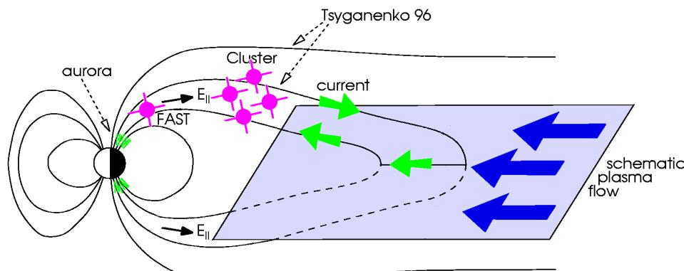
A schematic sketch of the auroral current circuit (adapted after Hamrin et al., 2006). Above auroral arcs, at about 1-2 RE altitude, the electrons are accelerated to keV energies by the parallel electric field inside the auroral acceleration region (AAR). Conjugated data from the Cluster and FAST spacecraft may be used to cross-check simulation results and probe the processes that lead to aurora.
