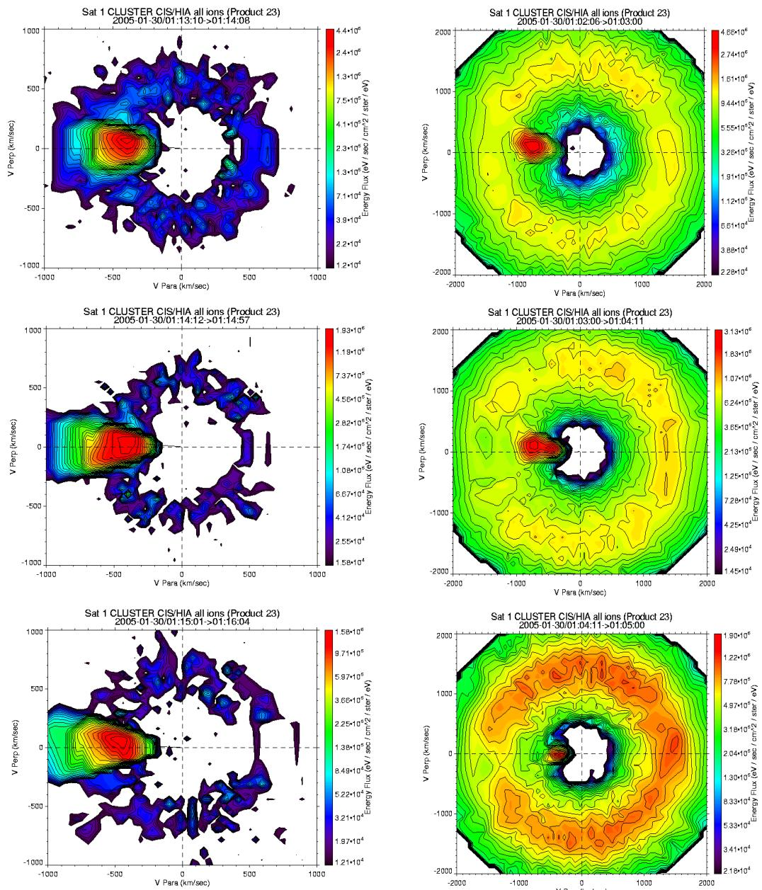
**Left:** C1 HIA distributions measured around the conjunction time of C3 with FAST, when C1 is a few latitude degrees away from the conjunction site. The distributions show a ~1 keV ion beam.
