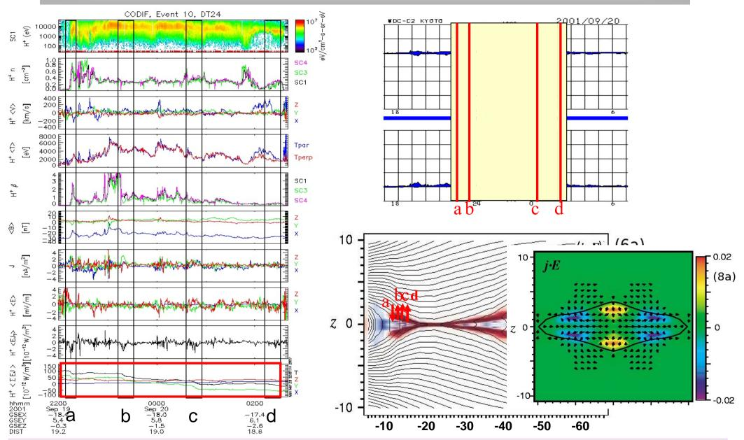
$\triangleright$  Although the average E.J shows load character [(x, z) panel], the local signature can still indicate a generator [(y, z) panel].
