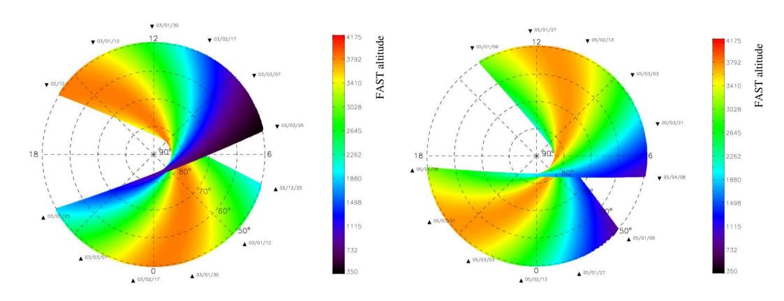
FAST altitude (color) as function of latitude and local time. The orbit rotation in local time is indicated by printing the date for a few orbits. The motion along the orbit is from the upward triangle to the downward triangle.
