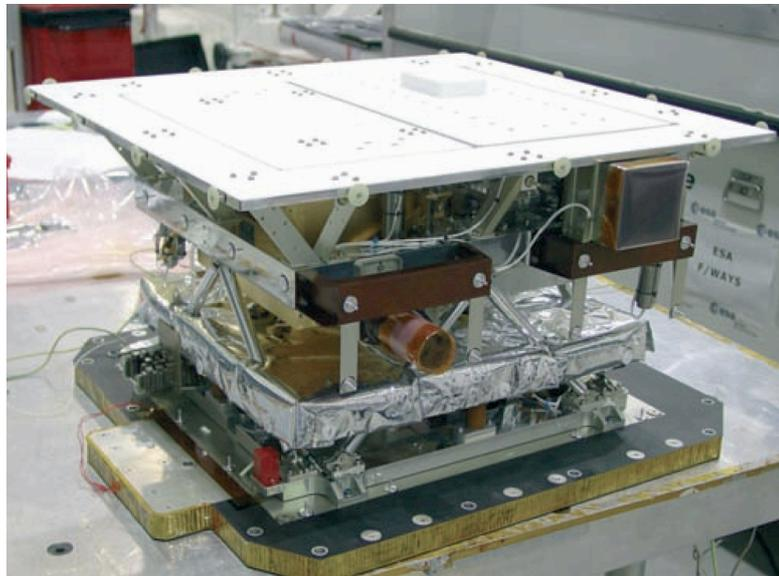
**Figure 6-3.** The optical module of the VIRTIS/Venus Express is a representative instrument, providing heritage for VIRHIS (Credit: INAF, LESIA)
