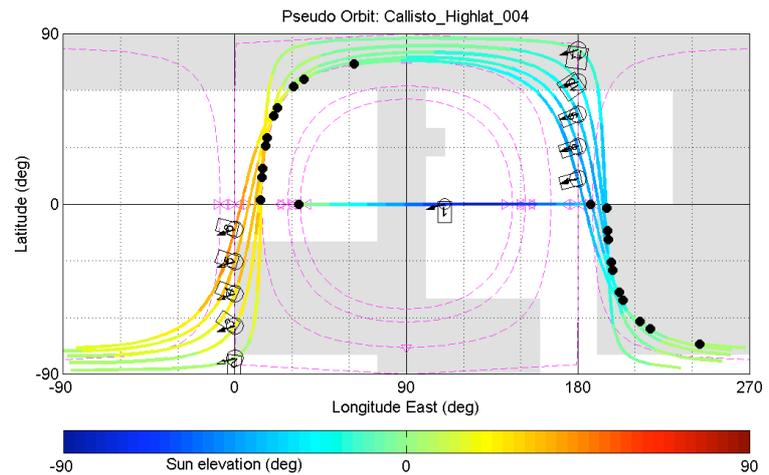
**Figure 7-6** Ground track of the Callisto flybys for altitudes <5000 km. The colour scale indicates local Sun elevation of the sub-nadir point in degrees (values <0° refer to local night). Numbers indicate the sequence of the flyby. The shaded areas correspond to gaps from Galileo and Voyager data. The black circles indicate closest approach, and the small arrows indicate the direction to the Sun.
