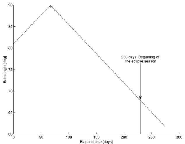
**Figure 7-9** Evolution of the sun declination ( $\beta$ -angle) as a function of time during the 200 km circular Ganymede orbit phase. The sun declination angle continuously changes, even after dawn-dusk orbit. The first eclipse is reached after 230 days from the start of this phase.
