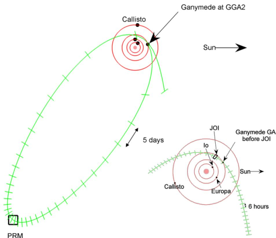
**Figure 7-1** Trajectory of the first Jupiter orbit. Also shown are the orbits of Callisto, Ganymede, Europa and Io. The inset shows the JOI together with the preceding Ganymede gravity assist.
