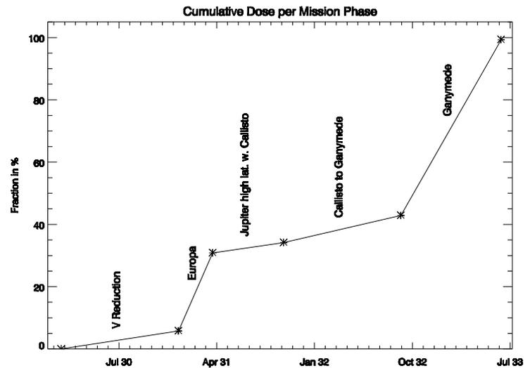
**Figure 7-12** Cumulative dose per mission phase. The figure shows the relative accumulation per mission phase as a function of time
