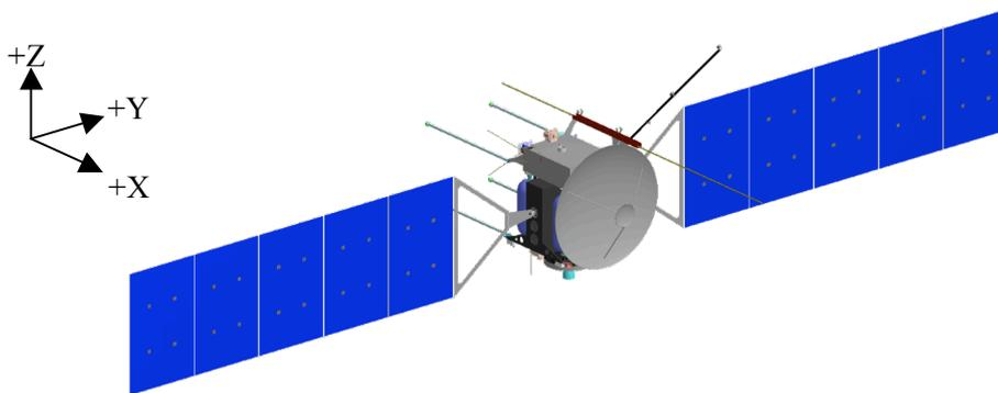
**Figure 7-18** Spacecraft configuration of solution 3. The main engine and the launcher interface are at the  $-Z$  side. The nadir direction is at the  $+Z$  side (up), and main component of the velocity remains parallel to the  $-X$  direction for all observing modes.
