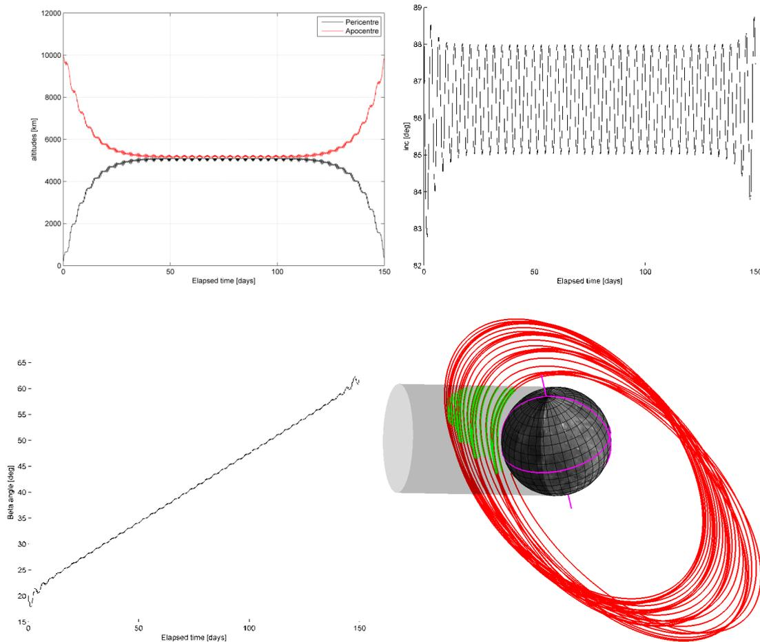
**Figure 7-8** Evolution of the orbit during the Ganymede elliptical and circular 5000 km phases: apocentre and pericentre altitudes (top left); osculating inclination (top right); sun declination, called  $\beta$ -angle (bottom left). On the bottom right the initial orbits following the Ganymede orbit insertion are shown together with Ganymede's shadow.
