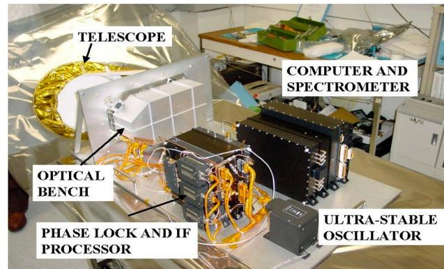
**Figure 6-5.** The flight model of the MIRO/Rosetta is a representative instrument, providing heritage for SWI (Credit: JPL, MPS)
