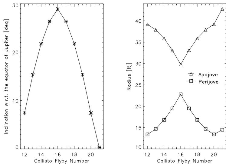
**Figure 7-5** Key properties of higher inclination orbits. The increase and decrease of inclination (left) and the apojove and perijove radii (right) are plotted as a function of the number of Callisto gravity assists.
