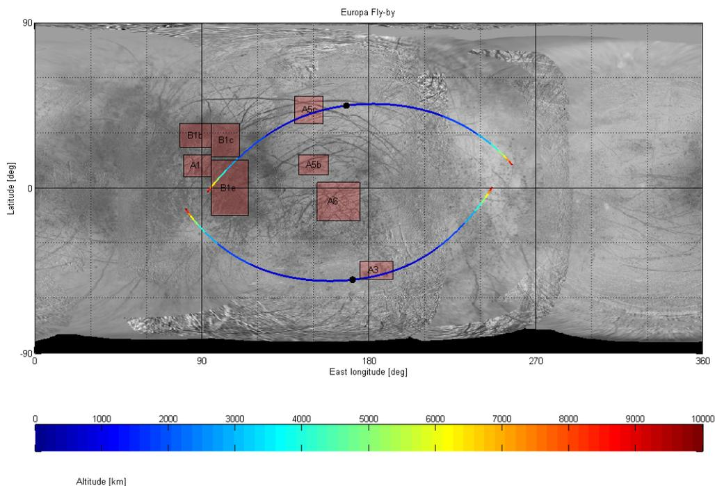
**Figure 7-3** Ground track of the spacecraft during Europa flybys. The image shows a Europa surface map with the areas of specific interest indicated by colour rectangles. The ground tracks of the two flybys are indicated in coloured lines, with the colour indicating the altitudes in 1000 km (see colour bar). The closest approaches are plotted by red dots.
