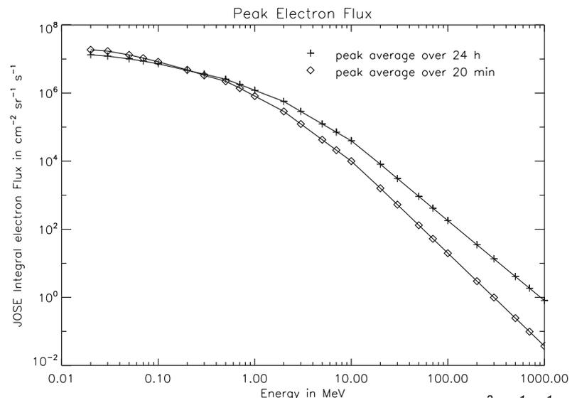
**Figure 7-13** Worst case integral electron flux spectra in  $\text{cm}^{-2} \text{sr}^{-1} \text{s}^{-1}$  during the Europa flybys, averaged over 24 h and 20 min.
