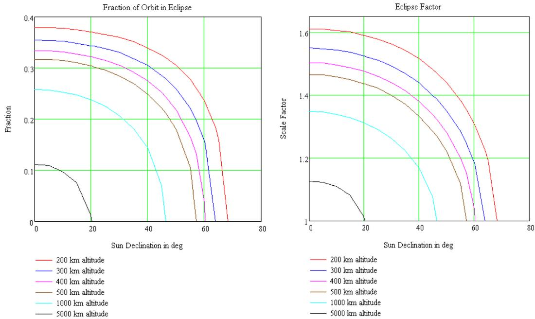
**Figure 7-7** Influences of eclipses by Ganymede on the spacecraft design. Left: the fraction of time spent in eclipse as a function of Sun declination to the orbital plane for circular polar orbits with altitudes from 200 to 5000 km. Right: the scale factor of increase of the solar panel area for additional power generation in compensation for the time in eclipse.
