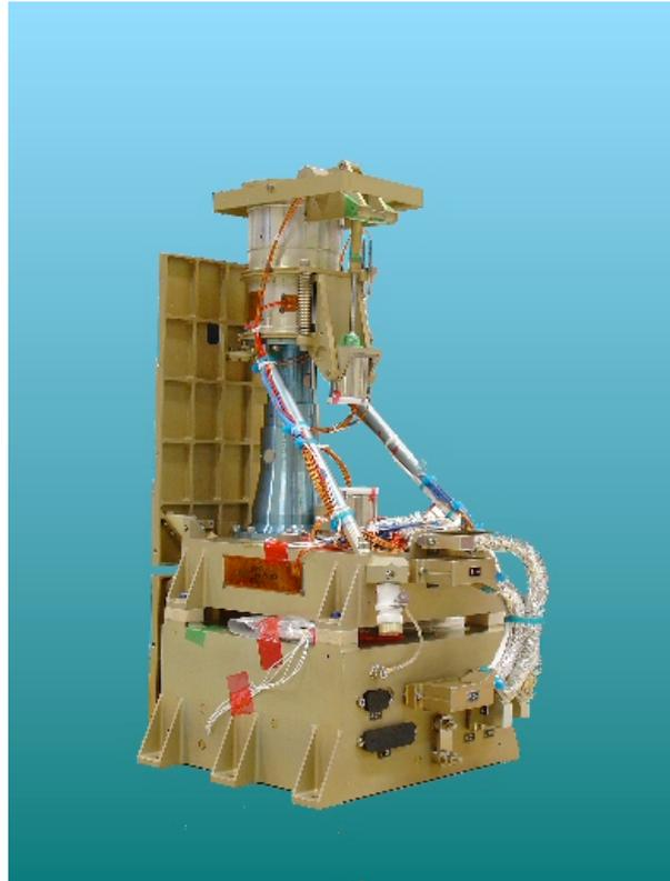
**Figure 6-1.** Framing camera for the DAWN mission is a representative instrument, providing heritage for NAC (Credit: MPS, DLR)
