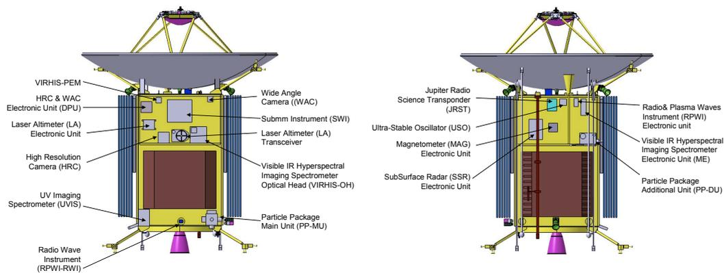
**Figure 7-17** Accommodation of the model instruments in spacecraft solution 2. Platform equipment would be accommodated within the volumes, which are indicated by brown covers in this drawing.
