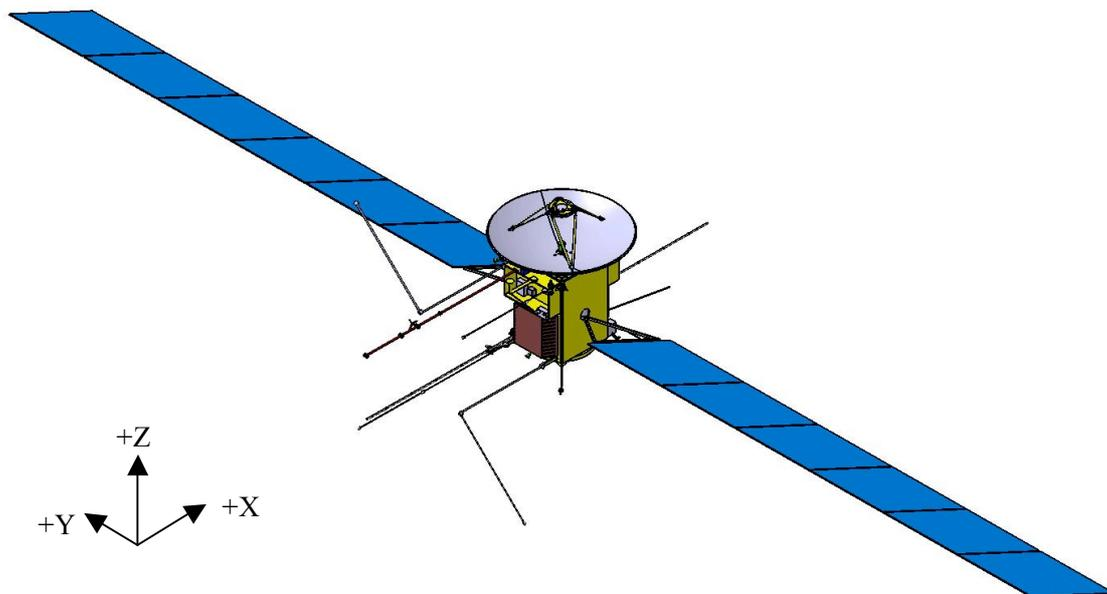
**Figure 7-16** Spacecraft configuration of solution 2. The main engine and the launcher interface is at the bottom (–Z panel), the remote sensing instruments are located at the back of this view (+X panel), and the in situ instruments, which require access to the velocity direction are mounted on the –X panel. The high gain antenna is at the top (+Z panel).
