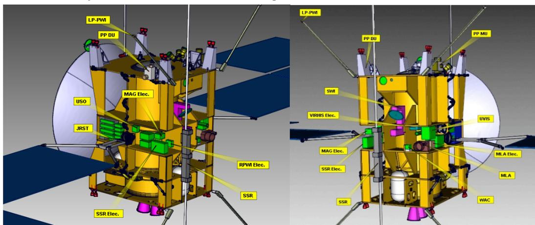
**Figure 7-15** Accommodation of the model instruments in spacecraft solution 1.
