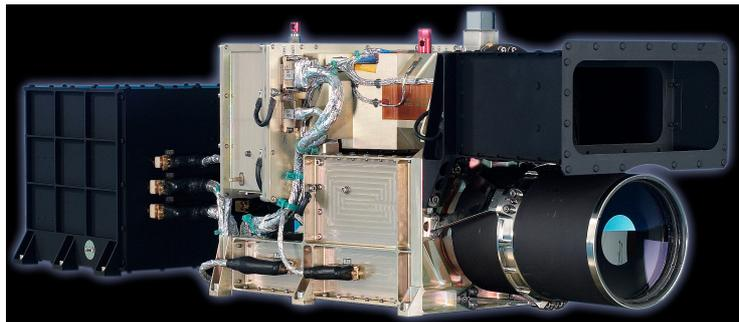
**Figure 6-2.** HRSC - SRC/Mars Express camera is a representative instrument, providing heritage for WAC (Credit: DLR, INAF)
