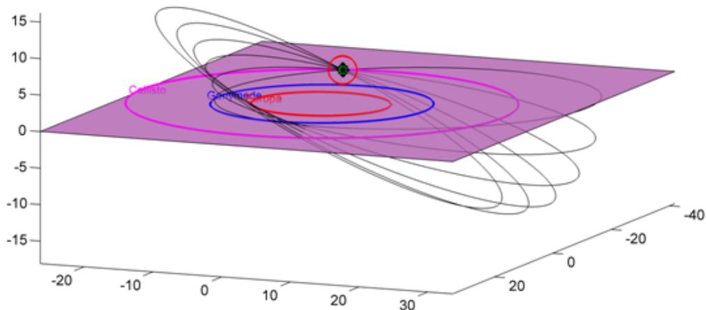
**Figure 7-4** The spacecraft trajectory (black) during the Callisto gravity assists to raise the orbit inclination. The Jupiter equatorial plane is indicated in pink, including the orbits of Callisto (purple), Ganymede (blue) and Europa (red). Jupiter is located at the centre (at coordinates [0,0,0]). Units are multiples of Jupiter’s radius.
