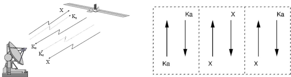
**Figure 6-12.** Triple link - X/X, X/Ka (Ka1) and Ka/Ka (Ka2) - operations proposed for JUICE
