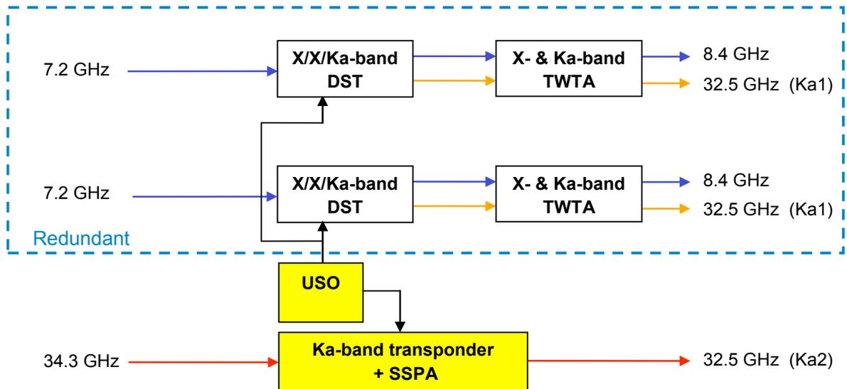
**Figure 6-11.** JUICE Radio Science payload (in yellow) integrated with the TT&C system
