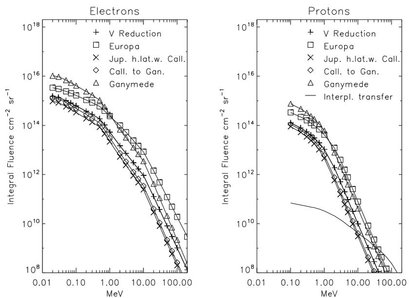
**Figure 7-10** Fluence spectra of electrons (left) and protons (right) per mission phase.
