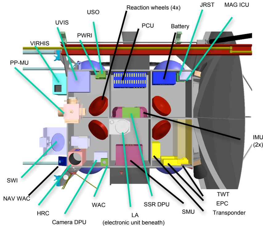
**Figure 7-19** Accommodation of the model instruments and platform units in spacecraft solution 3.
