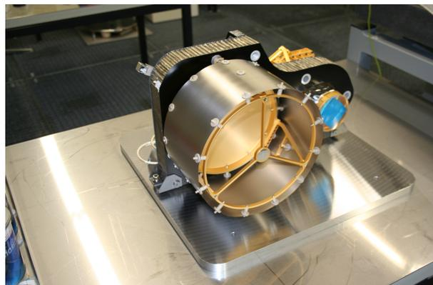
**Figure 6-6** Structural and Thermal Model (STM) of the BepiColombo laser altimeter BeLa is a representative instrument, providing heritage for the LA (Credit: BeLa Team UBE/DLR/MPS).
