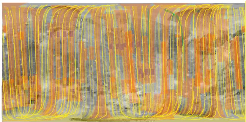
**Figure 5-6.** MAPPs simulation of JUICE surface coverage in the IR (orange), visible (yellow), UV (purple), and the penetrating radar (Green) after phase 8 (before circularisation at 500 km). Hyperspectral imaging at 2-3 km/px will be obtained over more than 50 % of Ganymede's surface. Imaging of the entire surface at 20, and 10 km/px will be achieved with the wide angle camera (not shown), together with several hundreds of very high resolution panchromatic images.
