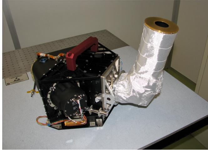
**Figure 6-4.** Structure thermal model of the Phebus/Bepi Colombo is a representative instrument, providing heritage for UVIS (Credit LATMOS)
