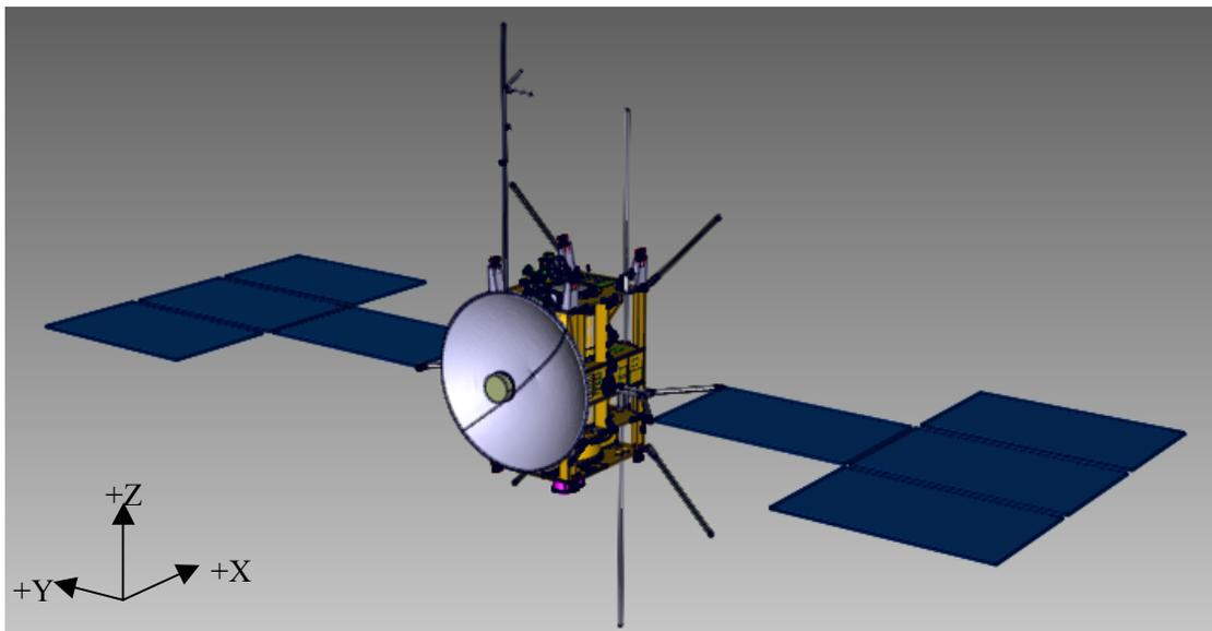
**Figure 7-14** Spacecraft configuration of solution 1 shown with the side panels removed. The main engines and the launcher interface would be at the bottom ( $-Z$  panel), the remote sensing and *in situ* instruments, which require access to the velocity direction would be located at the back of this view ( $+X$  panel). A cold plate would be at the top ( $+Z$  panel).
