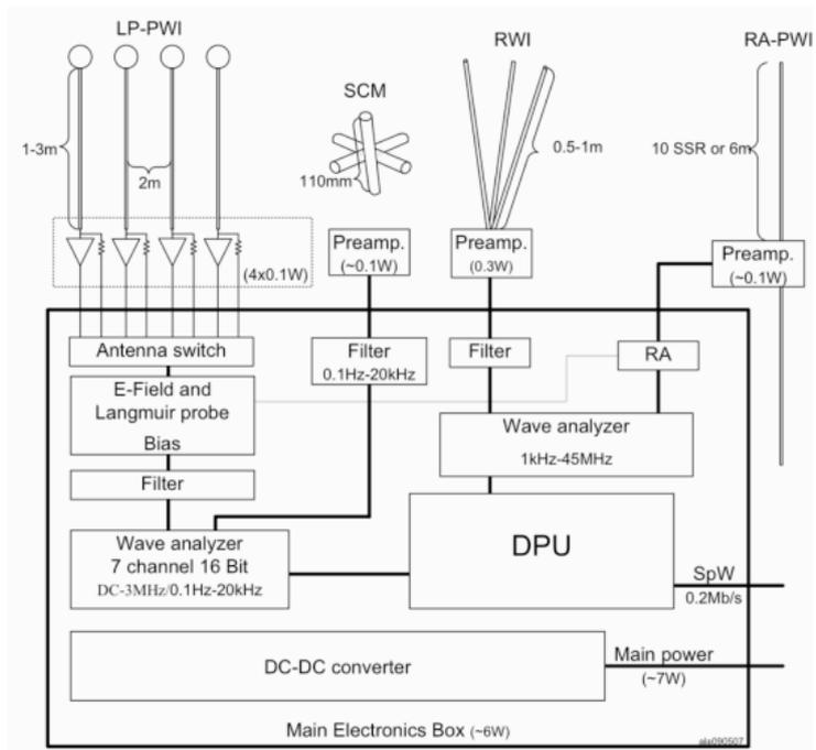
Figure 6-9. Block diagram of the potential RPWI instrument
