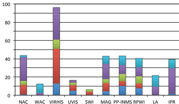
**Figure 5-1.** Example of data volume production (in Gb) by the model instruments [D-1] during the baseline Ganymede mission, and assuming D/L capabilities of 1.4 Gb/day. On each bar, the colours indicate the data volume per phase from bottom (phase 6) to top (phase 10). Circular phases at 5000, 500, and 200 km altitude are shown in red, purple, and light blue at the top of each bar, respectively.
