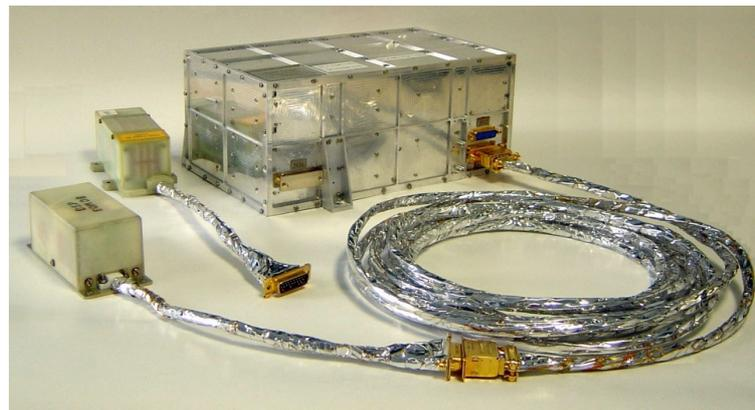
**Figure 6-8.** Double Star magnetometer, with electronic box, in and outboard sensors and boom cable, as representative instrument, providing heritage for MAG (Photo courtesy Imperial College).
