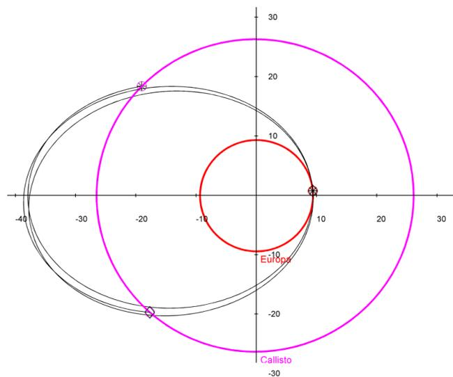
**Figure 7-2** Two Europa flybys from a 4:1 resonant orbit. The orbits of Callisto (purple), Europa (red) and the spacecraft (black) are drawn on a Jupiter Solar Orbital (JSO) coordinate frame. Symbols indicate the encounters of the spacecraft with the moons
