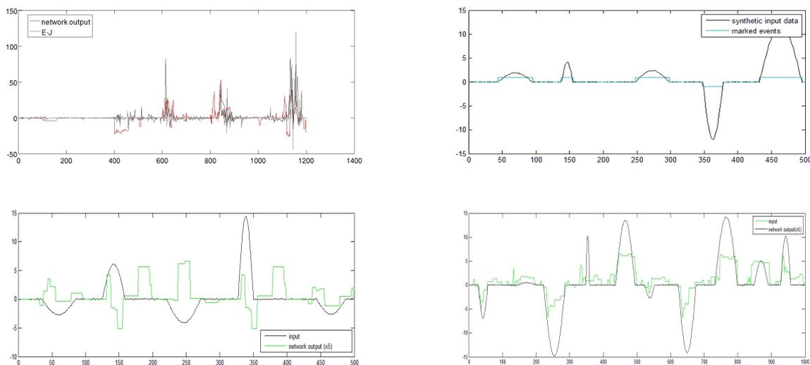
Figure 1: NN detection of real ECR events after training on Cluster data (top left), NN training on synthetic data (top right), and NN detection of synthetic ECR events (bottom left and right). The detection of synthetic ECR events is considerably improved in the bottom right panel, where the training set was larger, although the the NN had a smaller number of neurons.
