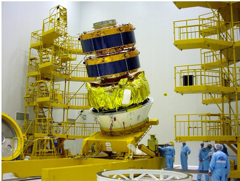
**Figure 2.1:** The second Cluster pair and the Fregat upper stage ready for integration into the Soyuz fairing. Location: The Upper Composite Integration Facility, Baikonur, Kazakhstan. Courtesy of ESA.
